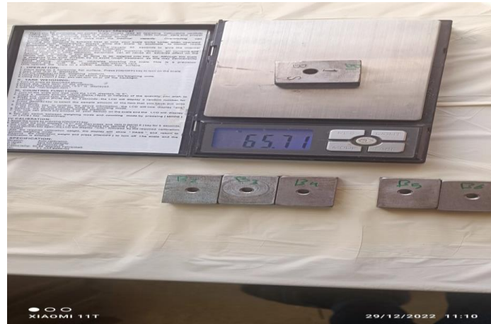
Fig. 6. Low carbon steel Sample weight
