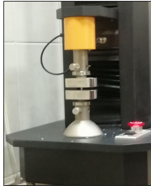
Figure (3) Compressive Strength Measurement by the Universal Testing Machine.
